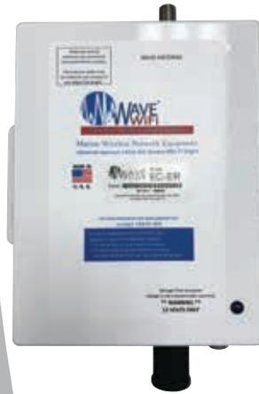
The EC ER comes with 25ft of LMR 400 cable that is then connected to a powerful High Gain Omnidirectional antenna giving the system an incredible amount of range. The system is a more cost effective mid-range solution when comparing our more powerful EC HP and shorter range Rogue systems.
